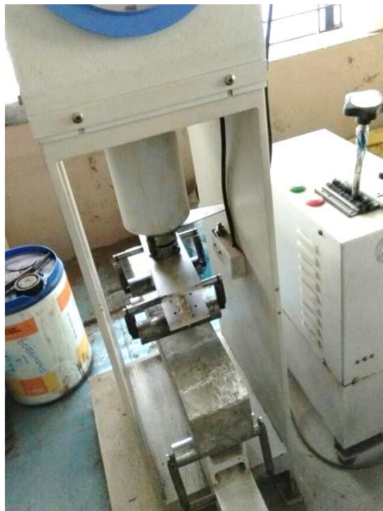
Figure 5. Flexural strength testing of fiber reinforced self-curing concrete
