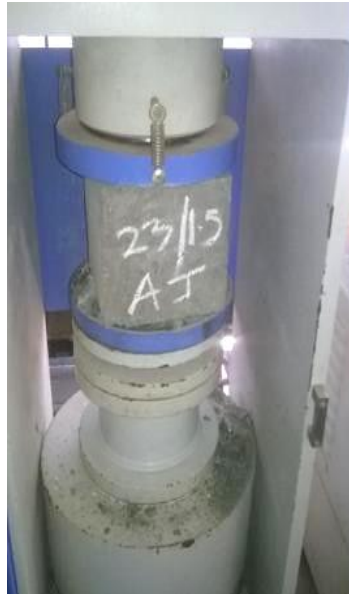
Figure 1. Compression test on a Fiber reinforced self-curing concrete cube
