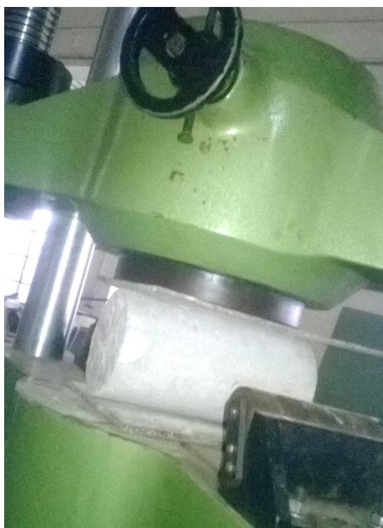
Figure 3. Split tensile test configuration for self-curing fiber-reinforced concrete.
