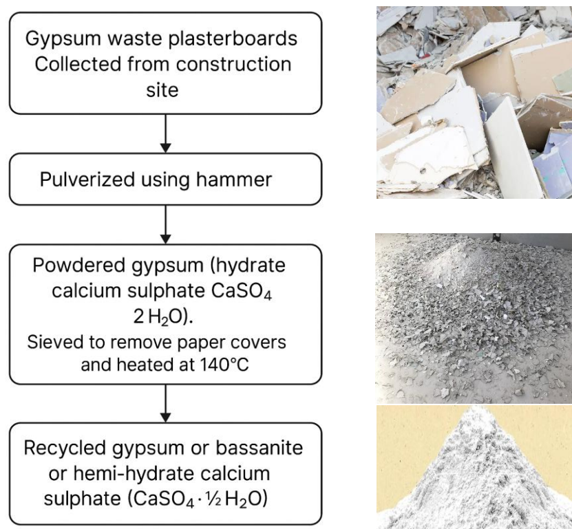
Figure 2. Procedure for the preparation of recycled gypsum
